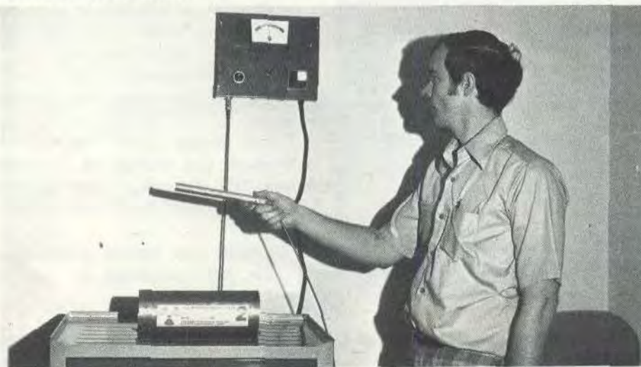
....John Milford, NAL Radiation Physics Section, checks a section of beampipe for induced radioactivity with the "Wallflower" probe....
