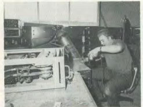
.... Roy Mraz working on assembly of an SCR module in service building D-0...
