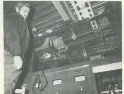
... Jim Garvey adjusting frequency of the nuclear magnetic resonance probe, in service building A2...
