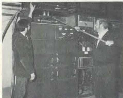
...(L to R) Pighetti & Garvey disconnecting a power supply from Main Ring magnet bus....
