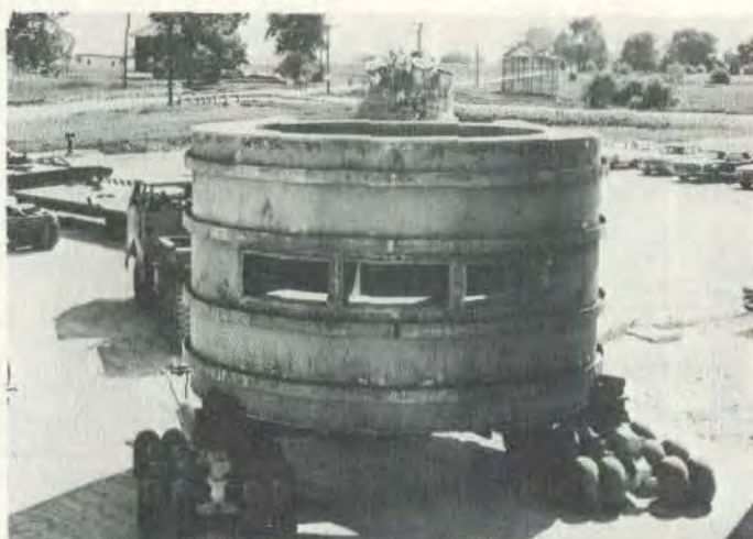
...150-ton superconducting magnet moved to its final location in the NAL 15-foot Bubble Chamber last May...
