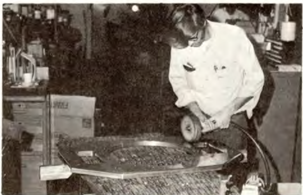
...Ralph Ovitt, Machine Shop, buffs part of Neutrino Horn...
