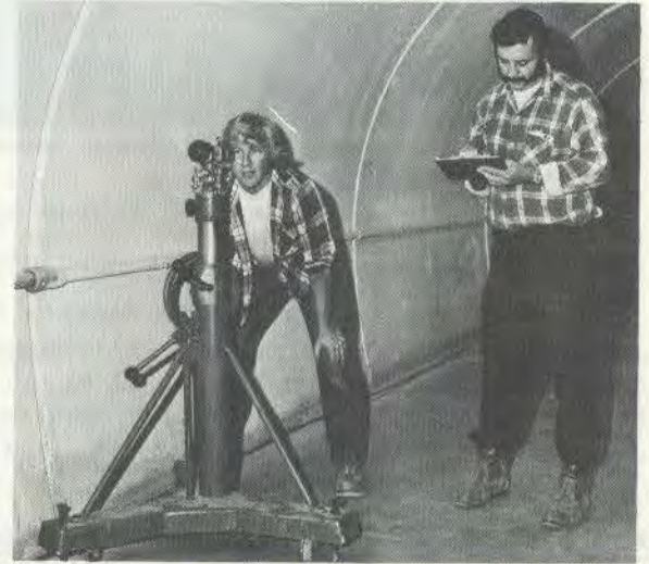
...Two members of the survey crew now measuring magnets of the Main Ring are (L to R) Frank Juravic and Ron Currier...
