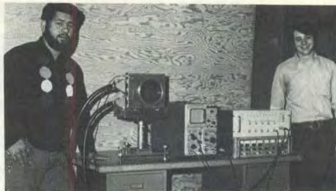
...Eddie Fuentes, trainee, and Steve Bjerklie with the SWIC and scanner they helped to build to monitor the proton beam in the Neutrino and Meson Laboratories...
