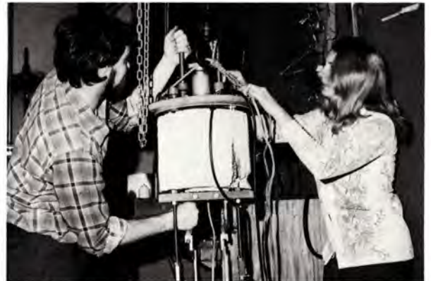
...Bob Pighetti (L), Peggy Price on a short sample test of Doubler conductor...
