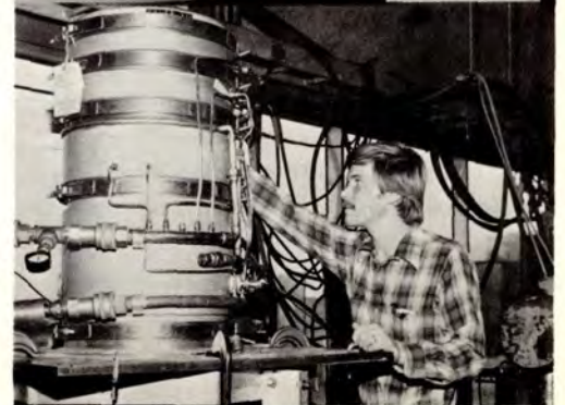
Since May, 1971, the Booster Accelerator has taken 200 million electron volt protons from the Linac and "boosted" their energy to 8 billion electron volts. They are then injected into the Main Accelerator. The Booster synchrotron is about 500 feet in diameter. Twelve "bunches" of Booster protons are required to fill the Main Accelerator.
