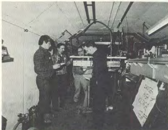
....Boyd Dean, Henry Koecher, Leonard Indykiewicz and Ed Hubbard administer power tests to septum magnet in Booster ring....
