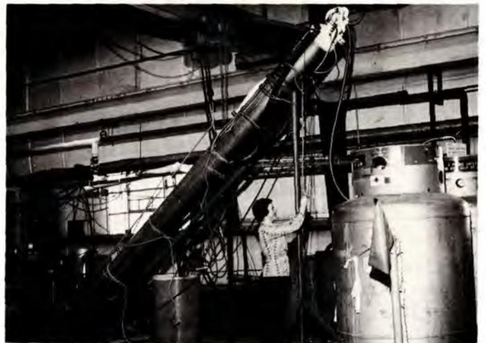
...Louise Latreille adjusts cable for C2-10 test. Cryostat containing magnet is in diagonal position...
