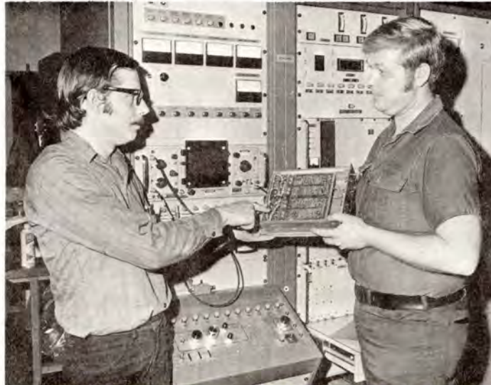
...(L-R) Wayne Ganger and Gerry Erickson examine an automatic frequency control module at the control system of one of the nine RF systems in the linac...
