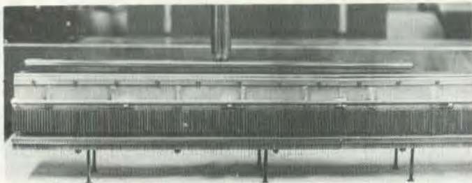
...The electrostatic septum which pulls the proton beam out of the Main Ring so that it can be directed to experimental areas...
