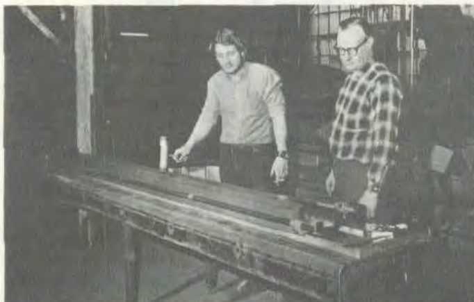
....AT THE SANDERSON PLANT: Bob Kreml, NAL Main Ring, resident inspector, (right) watches as Dick Hanson, Technician, works on assembly of Beam Transfer magnet half-cores....
