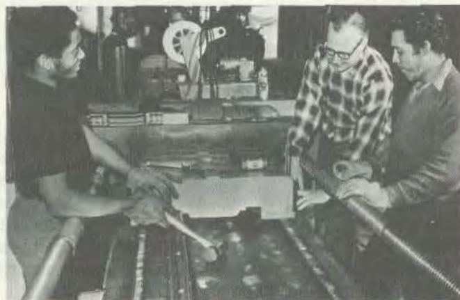
....Charles Sanders, Bob Kreml and German Olmos (l. to r.) at stacking of B-1 magnet half-core in Chicago South Side plant....
