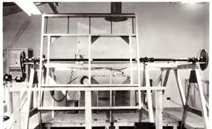
...Detector Development group's new winding device in operation. Completed wire winding may be seen faintly on the right portion of the frame...
