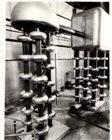
Cockcroft-Walton generator for new negative ion source.
