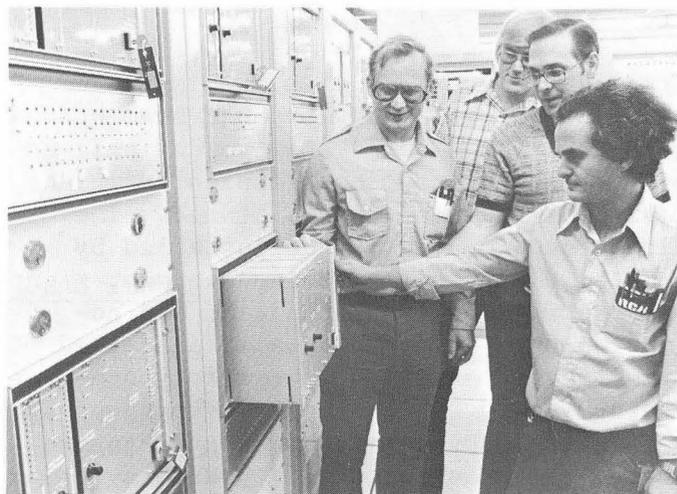
...In the Meson Area control room, (left to right) Paul Czarapata, Glen Federwitz, Jerry Dyche and Skip McGuire examine the M-4 beam line safety control chassis. The M-1 chassis is at the extreme upper left of the photograph (the one with the key and tag). Just below it is a chassis that services the M-1 chipmunks. At the bottom left of the photograph is the system for the M-2 beam line...
