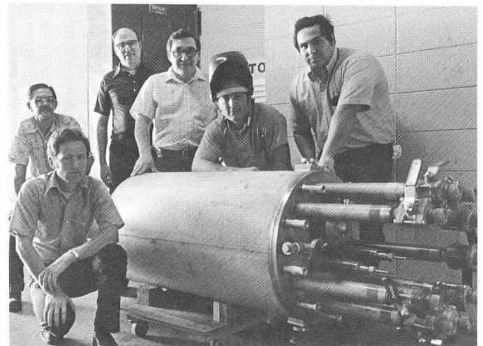
Valve box. Its function is to integrate the flow of liquid helium from the satellite refrigerator and the Central Helium Liquifier Facility along with liquid nitrogen. They are sent along the tube at the left of the photograph to the superconducting magnets. The liquid nitrogen provides the shield cooling and the liquid helium bathes the magnet coils, keeping them at superconducting temperature. From the left are Bill Noe Sr., John Colvin, Carl Pallaver, Ernie Ramirez, Rich Krause and Gerry Kusiolek.
