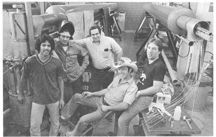
Two heat exchanger trains. Others similar to these can be seen protruding from the buildings on top of the Main Ring berm at A3 and A4 (across from the industrial building complex). The exchanger trains shown here are being assembled. From the left are Ralph Afanador, a summer employee, Rich Krause, Gerry Kusiolek, Jim Thompson and Dave Hanabarger. The heat exchangers cool the high pressure gas from the compressors by using the low pressure cold gas returning from the magnet string in the tunnel.
