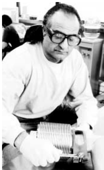
Fabricating the Recycler beam pipe, Chander Sood aligns a bellows and pump preparing for the tack weld...
