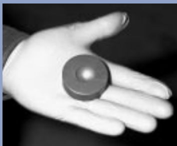
A beryllium window for a lithium lens.
