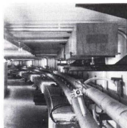
The Recycler, at the top of the photo, needs no power, cooling water, or fancy control systems to run.
