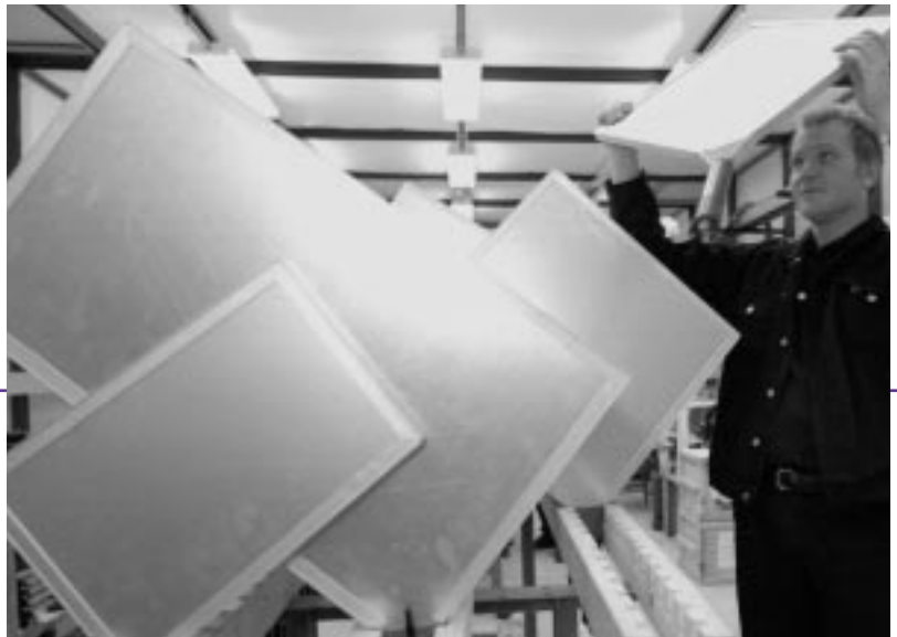
Russian physicist Andrei Schukin looks over a muon panel for the DZero detector.
