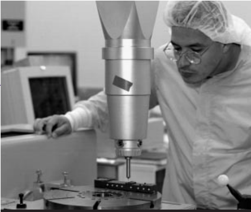
Precision silicon technology has a large role in both detectors' upgrades. Technician Jorge Montes uses a coordinate measuring machine in the Silicon Detector Facility.
