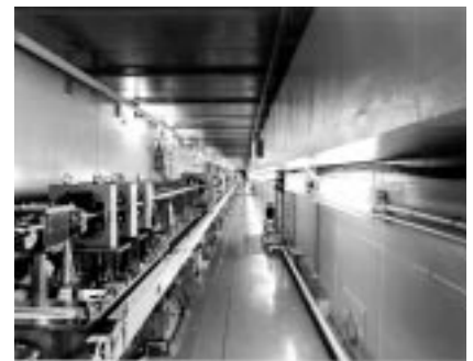
KEK's Accelerator Test Facility for a possible future NLC consists of two major components, including the 1.5-GeV injection linac shown here and a damping ring.
