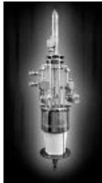
Prototype of a klystron for a future U.S. NLC. Klystrons are microwave tubes that use the same technology as airport radar and microwave ovens, but provide far more power.
