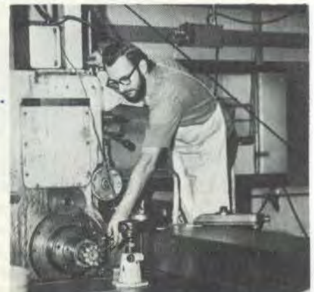
...Jerry Peterson boring aluminum parts on the King Vertical Boring Mill -- Village Machine Shop...
