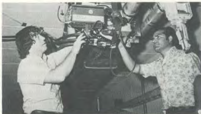
...Al Guthke and Jesse Guerra work on a scintillator screen and T.V. camera in the Proton Beam Line...
