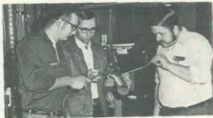
....(L to R) Tony Rader, Richard Applegate and Jack Johnson preparing the nitrogen shield for the long liquid helium transfer line....
