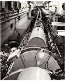
...Linear accelerator provides beam in CTF...
