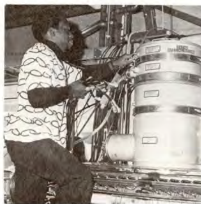
...Ruffin installing completed R.F. power amplifier on Booster test cavity...
