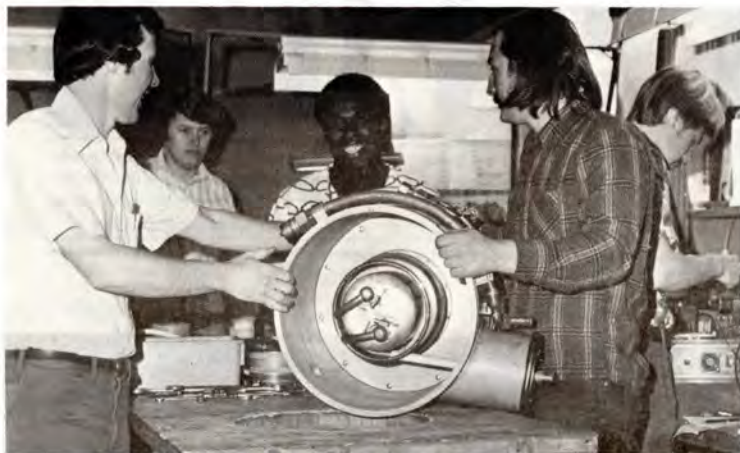
...Installation of new screen capacitor in R.R. power amplifier module. (L-R): Sarver, Tim Gierhart, Ruffin, Barnett, Bill Swedberg...
