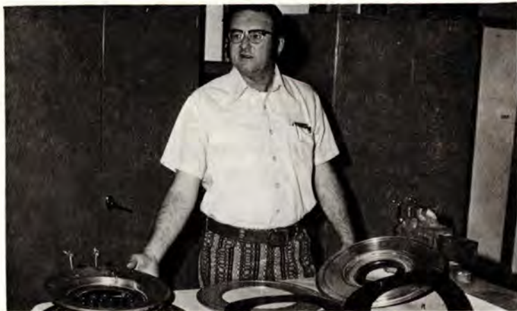
...Bill Miller points out the simplicity of new Kapton screen capacitor design, at right, over complex old model at left...
