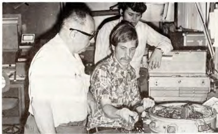
...Swedberg (seated) explains re-wiring of cascode driver module of the R.F. power amplifier to Carl Maier (L) and Gierhart...
