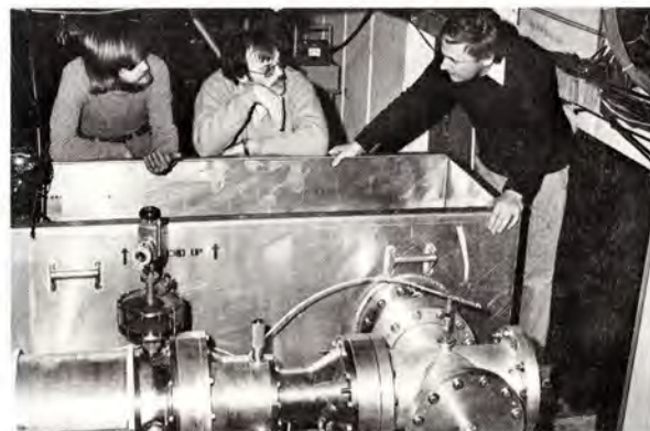
...B. Robinson, A. Jonckheere, H. Lubatti discuss capacitor changes in the Marx generator box...
