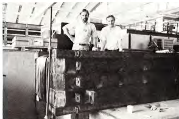
...J. Klems, H. Lubatti at the SOD magnet after experimenters have finished winding 101 turns on the iron in an all-night session...
