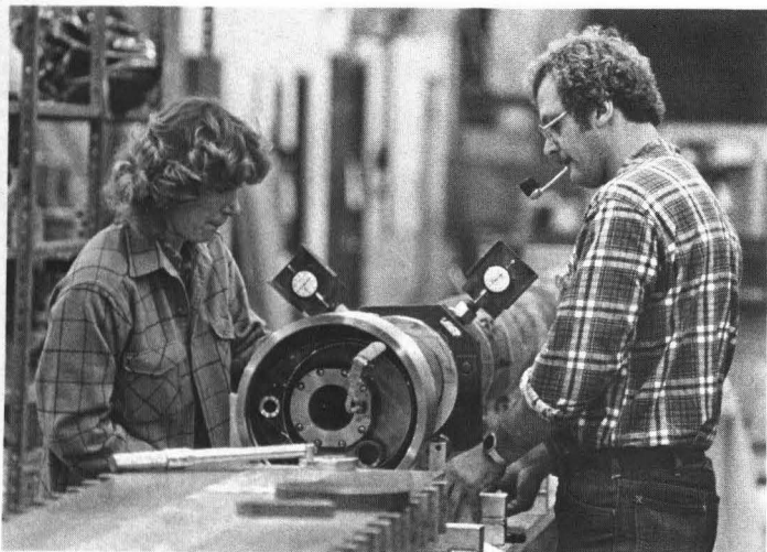
...Jo Gordon (left) and Bill Brudi, both inspectors, conduct a suspension measurement test on part of a cryostat...
