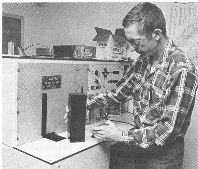
Jay Baldwin places a sample in the automatic sample changer. The germanium gamma ray detector and associated controls are in the unit in front of Baldwin.
