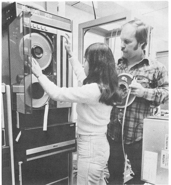
Ignacia Cuevas and Jim Meadows prepare to test one of the new 6250 bpi tape drives before delivery to a data acquisition computer for one of the high energy physics experiments.
