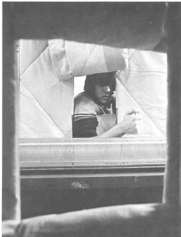
Greg Meyer applies silicon rubber to septum wire withdrawal springs while shielded by lead blankets.
