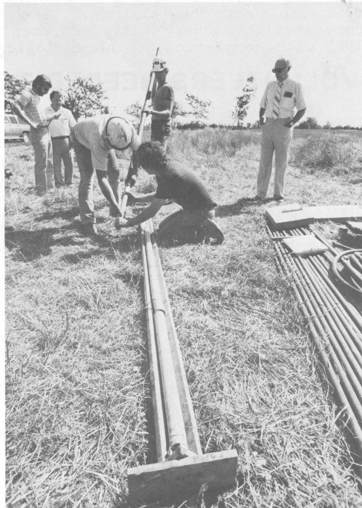
State Geological Survey team removes 10-ft long bedrock core with assistance from D&G Drilling, Inc.
