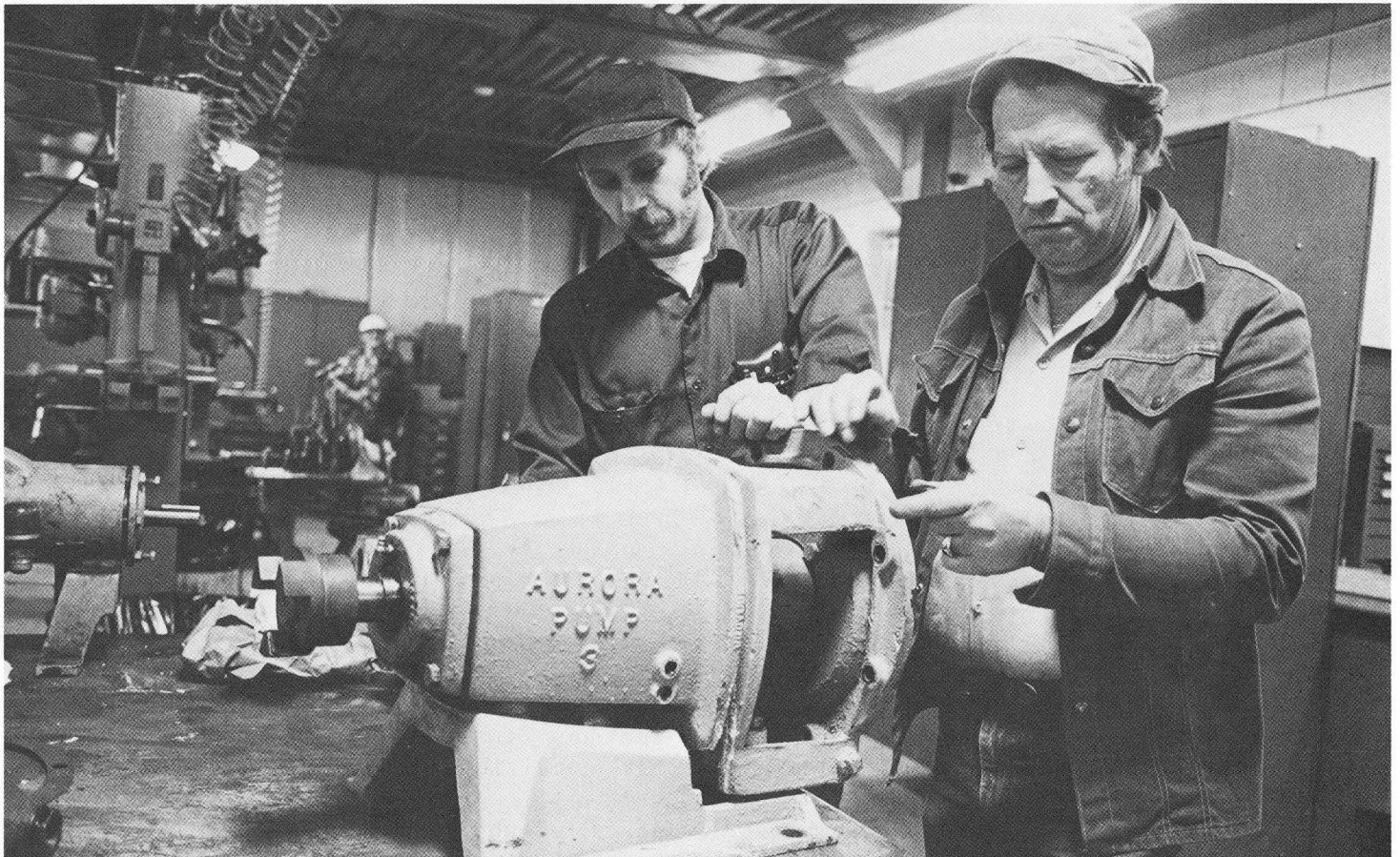
Ken Lindberg, left, and Don Walker repair a water distribution pump in the Maintenance Shop.
