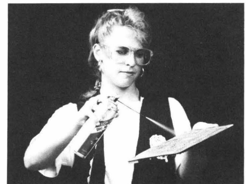
Aimee Vessell (ES&H) cleans a circuit board using an environmentally friendly cleaner. The committee has eliminated the use of Freon 113, previously used on circuit boards, because of its adverse effects on the ozone.
