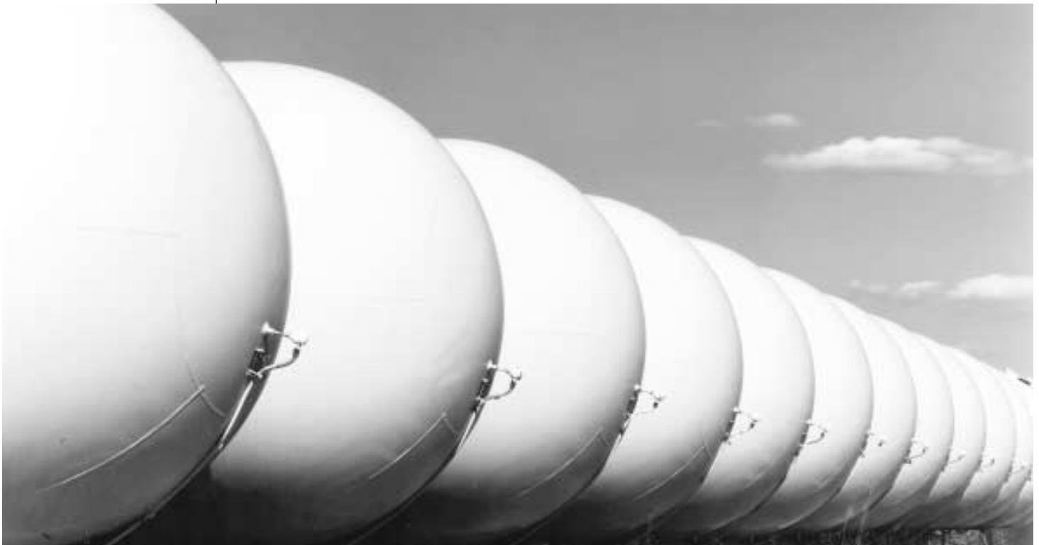
These 30,000 gallon tanks store gaseous helium at pressures up to 200 psi. The helium will be liquefied and used to chill the superconducting Tevatron, the world's most powerful accelerator.
