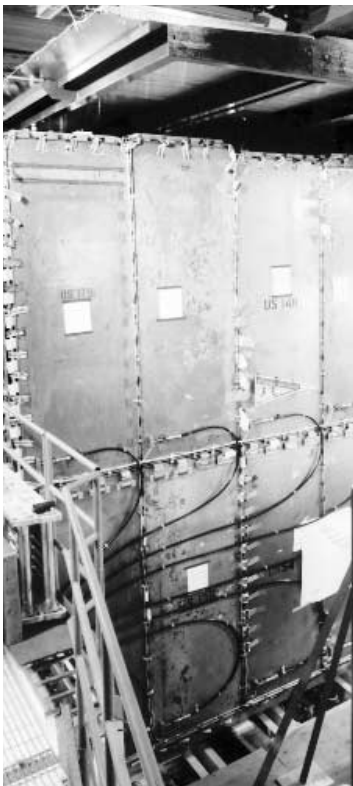
A 1-kiloton detector in an underground mine in Minnesota is now employed in the study of atmospheric neutrinos. It will be modified for use in the MINOS experiment.
