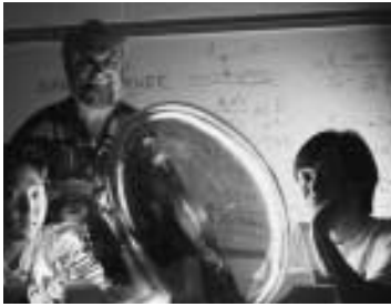
Physicists John Learned (standing), Shigenobu Matsuno (right) and Dean Takemori, of the University of Hawai'i, display a photomultiplier light detector, like one of the thousands lining the Super-K neutrino detector tank.
