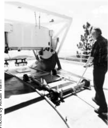
Carl Lindenmeyer rolls the cart in place to change the mapping cartridge on the telescope at Apache Point.
