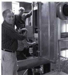
Chuck Schmidt invites you into the Cockcroft-Walton pre-accelerator, beginning the journey from hydrogen gas to proton beam. Jim Wendt and Ray Hren do some fine-tuning inside the apparatus.
