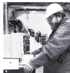
Jim Holub tests for leaks in the vacuum system.
