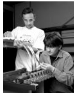
In Lab 5, fiber assemblies (pictured on the cover) for the hadron calorimeter scintillator systems are glued together by technicians Dan Ruggiers and Jaska Gielata, both of the University of Rochester.
