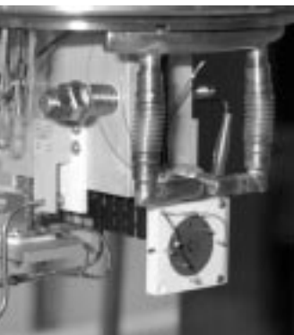
A prototype of the NuMI target, where proton collisions begin the production a neutrino beam. Note the comb-like configuration of the graphite target.
