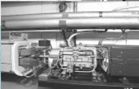
Main Injector Sector 10, showing focusing, corrector and steering magnets.
