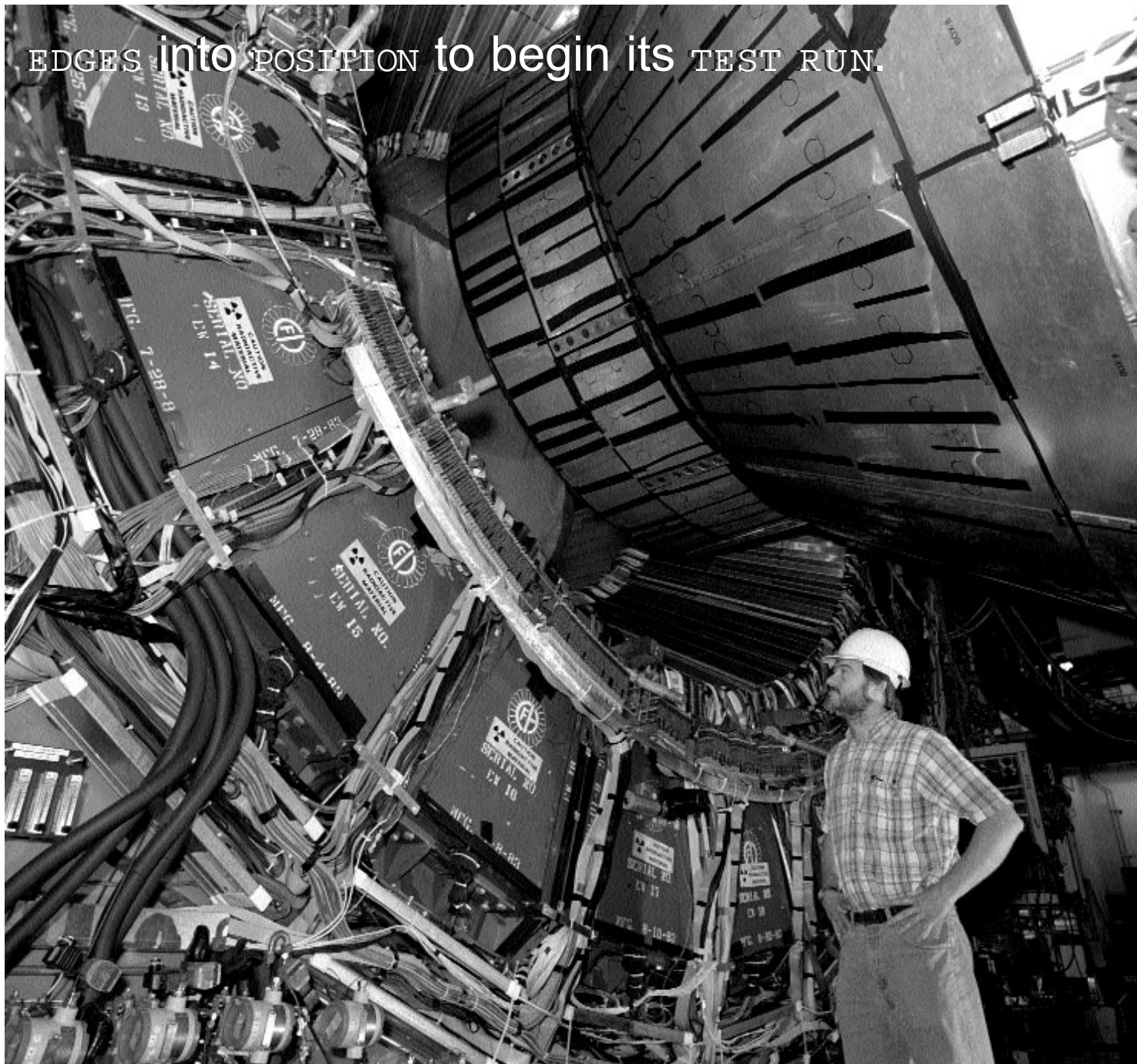
Fermilab physicist Pat Lukens inspects the proper positioning of one of CDF's two end caps inside the detector.
