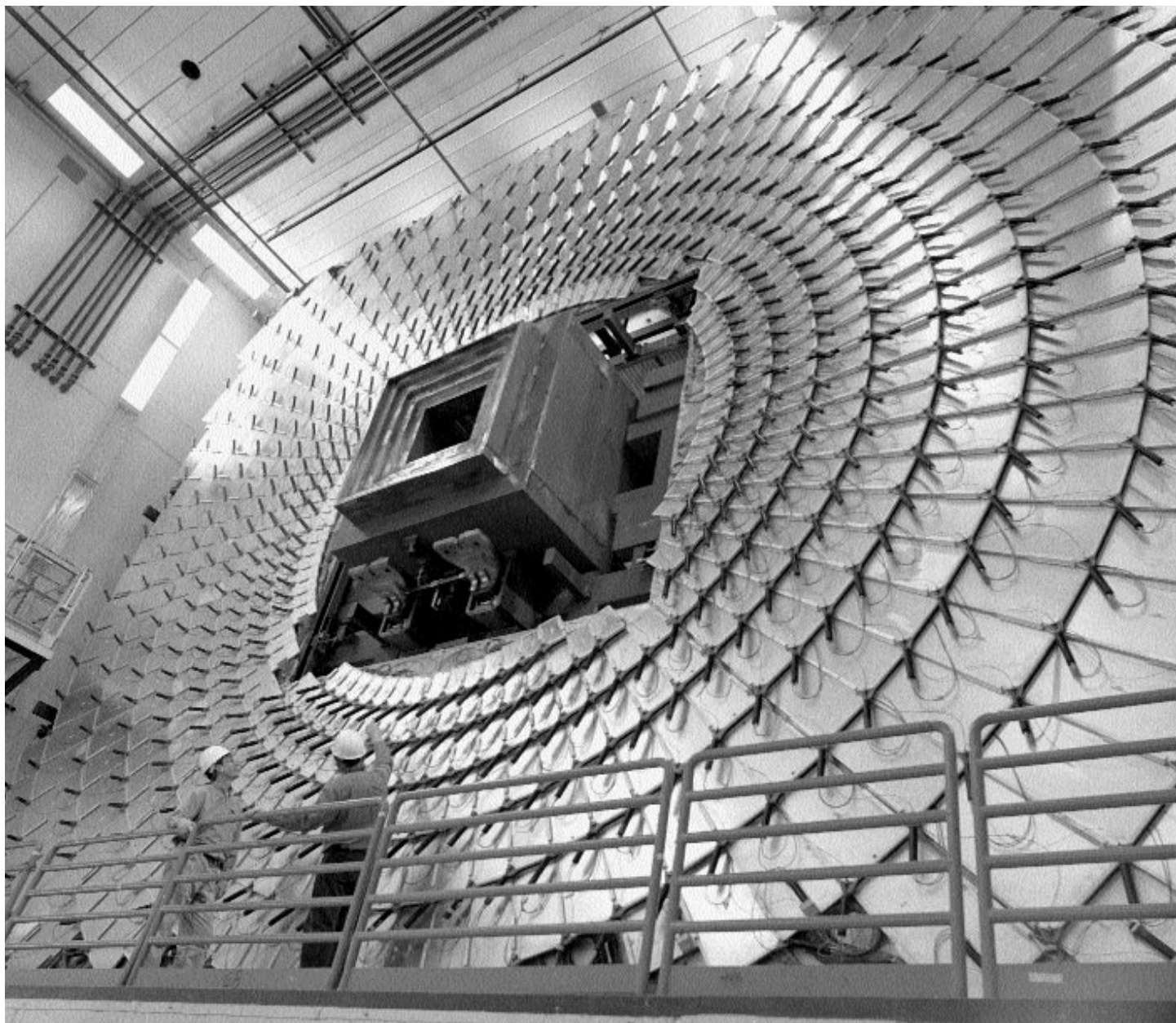
The 150-ton C-layer muon truss, part of the DZero detector, installed in the assembly hall. Above, time-lapse shots of CDF rolling into the beamline for a commissioning run.
